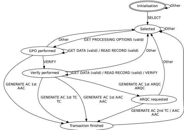
Fig. 4. Automaton of Dutch SecureCode Aut application. Note that here the `VERIFY` operation – i.e. verification of the PIN code – must be passed successfully before cryptograms can be generated, except for the AAC cryptogram to abort the session.
