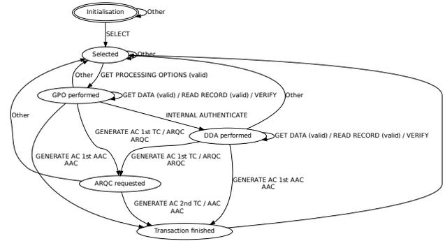
Fig. 3. Automaton of Dutch Maestro application. Just to highlight one observation that can be made from this diagram: the `VERIFY` operation, i.e. the verification of the PIN code by the smartcard, is optional; this makes sense because the terminal may check the PIN code with the bank (so-called online PIN verification), or choose not to verify the PIN at all.
